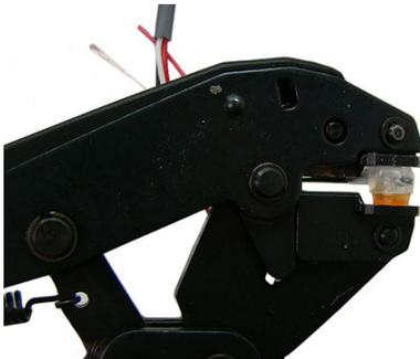
3. Squeeze the handles to crimp the connector. Apply pressure until the cap is fully seated (at least three seconds).
